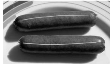
Figure 4.31. Hot dogs are cylindrical vessels pressurized with steam. Since the hoop stress is twice the axial stress, the dog's skin splits along its axis.
