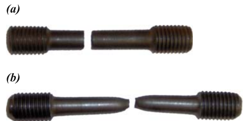
Figure 9.2. (a) Failure of a brittle (cast iron) tensile test specimen (0.5 in. diameter). Little plastic deformation occurs; the failure surface is flat. (b) Failure of a ductile (steel A36) tensile test specimen. Large plastic strains and necking occur before failure.
